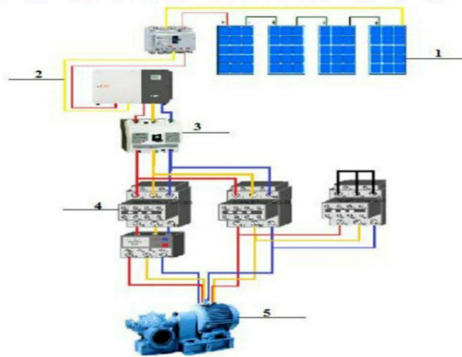
1-rasm. 1-quyosh panellari, 2-invertor, 3-uch fazali avtomat, 4-magnit ishga tushirgich, 5-nasos agregati.
